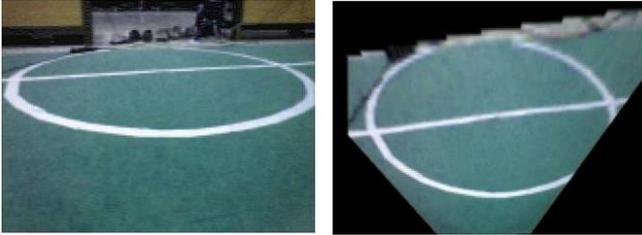
Fig. 8 Inverse perspective transform view of field
