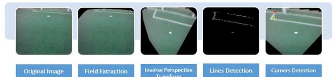
Fig. 6 Detection of field, lines and corners
