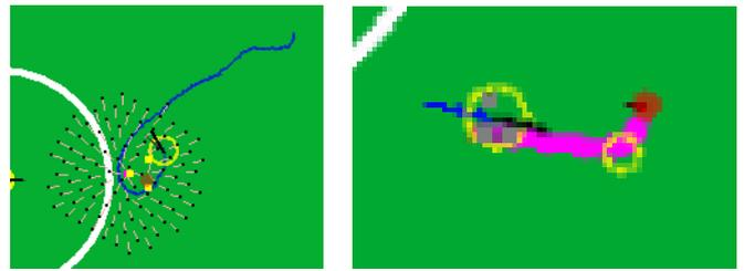
Fig. 10 Motion: Potential Field (left); Footstep Planning (right)
