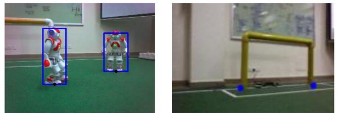
Fig. 7 Robot Detection (left); Yellow goal post base points (right)
