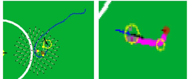
Fig.5 Motion: Potential Field (left); Footstep Planning (right)
