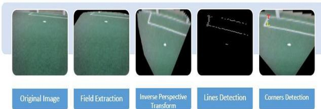
Fig.2 Detection of field, lines and corners
